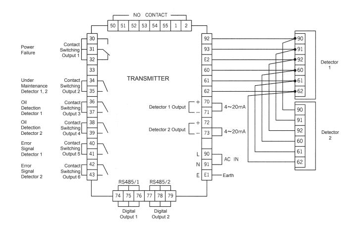
Detector 2 Connects to Terminals of Detector 1
